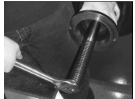
Figure 6 - Tighten the 40 mm Conversion Shaft
