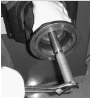
Figure 1 - Remove Existing Stub-Shaft
