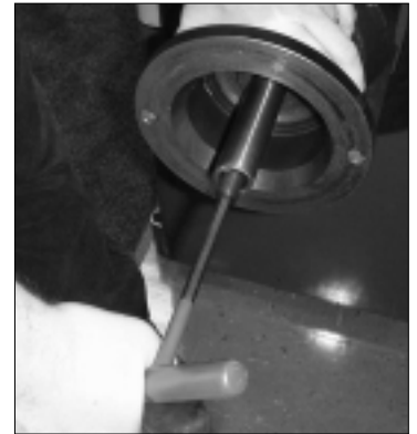
Figure 3 - Install the Coupler
