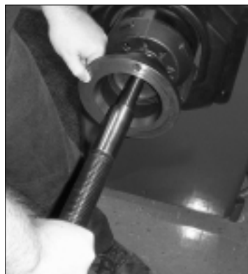
Figure 5 - Rotate to Engage Coupler Threads
