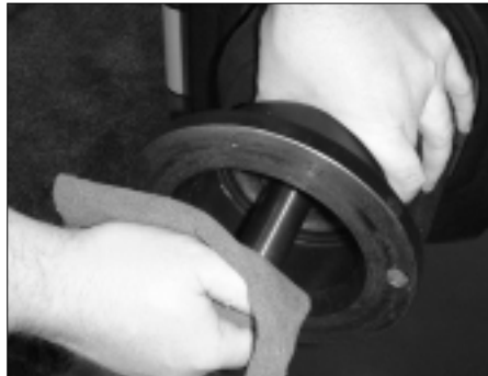
Figure 2 - Clean the Motor Shaft
