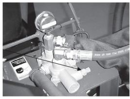
If the valve "kicks out" on the arms return stroke, the detent will have to be tightened slightly. Loosen lock nut as shown. Tighten outer nut 1/4 turn and tighten lock nut. Continue to crush. If it "kicks out" again, readjust it another 1/4 turn.
