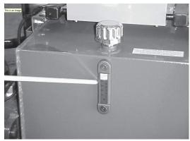
Check hydraulic oil reservoir level by viewing the sight glass. Oil level should be approximately 3" -5" from the top.
