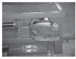
This photo illustrates the wheel being fully crushed.
