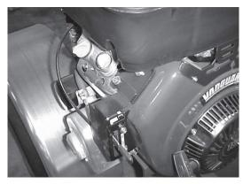
When crushing wheels, run engine at 3/4 open throttle.
