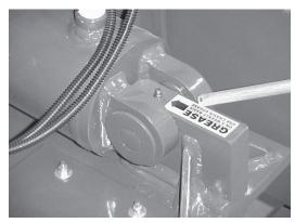
Periodically insert grease at the cylinder pivot.
