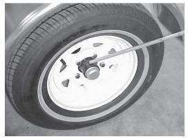
Once every 6 months, remove wheels & hubs from axle and pack the wheel bearings with a wheel bearing grease.
